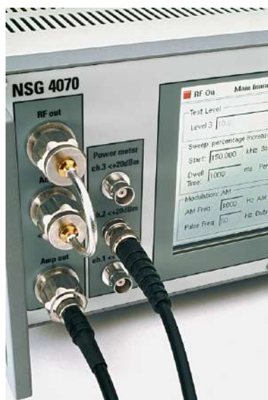
NSG 4070C1-LFCP front panel with RF ports
