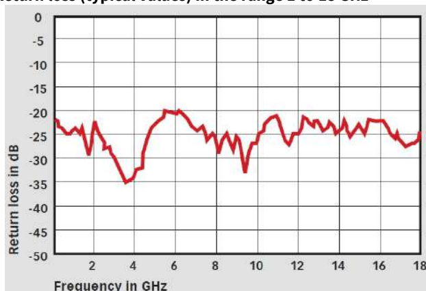
Return loss (typical values) in the range 1 to 18 GHz
