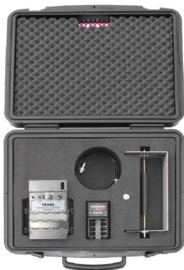
CVP 2200A, battery charger, calibration jig, RF cable and 50 Ω termination in suitcase
