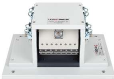
CIP 9138 with PCJ 9202 calibration jig
